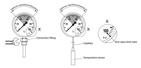
The temperature measuring point should be prepared according to the specifications for screw-in holes or thermowells. Further instructions can be found in VDE/VDI guidelines 3511 and 3512 sheet 2. Sealing washers to DIN 7603A are suitable for sealing. The correct tightening torque depends on the material and shape of the seal used. It should not exceed 80 Nm. When screwing in and unscrewing temperature gauges, do not tighten on the housing, but only on the wrench flats of the connection fitting.
